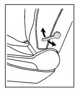
If your vehicle has this feature, the handle is located on the outboard side of the seat.
